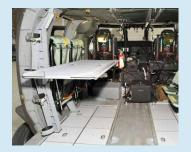
Hinged litter platforms and support arms easily remove for storage in the integrated box outboard of the AP Seats.
