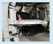
The litter slides onto platform via channels ensuring smooth and safe loading. Platform is then returned to flight position and locked for taxitakeoff-landing.
