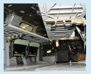
Track style mounting is provided under the upper platform, on the base pallet, and on the aft stanchion for mounting restraints, utility equipment, and medical IV bags.
