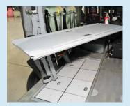
Litter platform is secured on support arms that telescope and rotate, allowing crew to change the angle and position of the platform.
