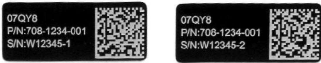
Figure 8: IUID Multiple Parts Part Mark Example
